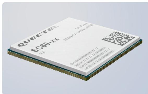
SC60 is Quectel’s new generation of multi-mode Smart LTE Cat 6 module with built-in Android 7.1 Nougat OS. Based on Qualcomm Octa-core and 64-bit high-performance processors, SC60 is designed to support leading performance, rich multimedia features and Quick Charge 3.0 technology. It is ideal for both industrial and consumer applications requiring high data-rate and multimedia functions.
