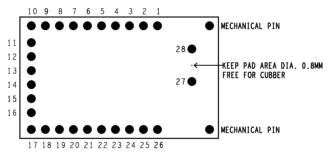
Figure 3: Module pin-out (top-view)
