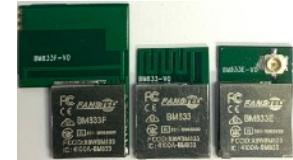
BM833/F/E, nRF52833 modules have compatible footprint for upgrading. They offer more GPIOs, more memories, +8 dBm TX.
